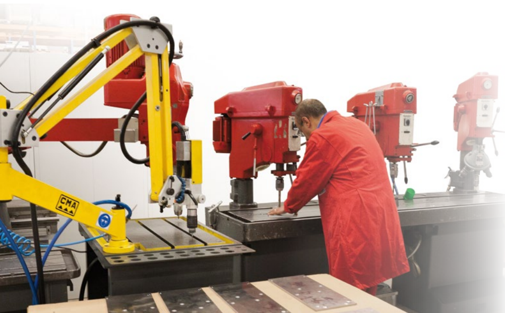
Combination of five processing steps: (From the right) Drilling, countersinking, counterboring, countersinking for thread-cutting and finally thread-cutting, all in one go.
